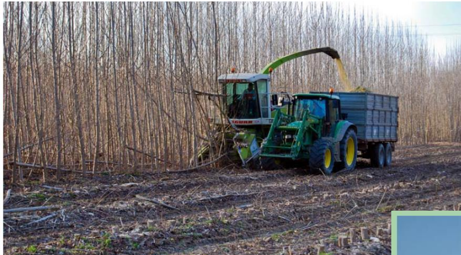
A modified self-propelled forage chopper cuts the poplars, makes woodchips and blows the chips into a trailer (Photo: L. Corbella & M. Cocchi, ETA)
