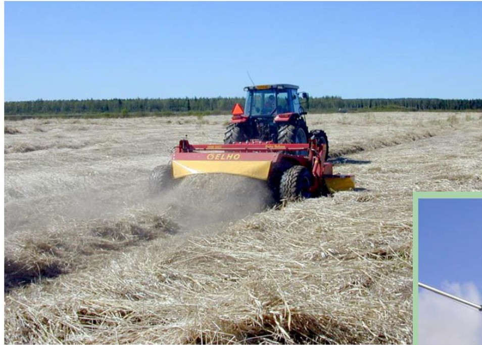
Disc mower with conditioner mowing RCG in spring. The snow has pressed the crop very near to the soil surface. It is important to set stubble height as short as possible. (Photo: Timo Lötjönen, MTT)
